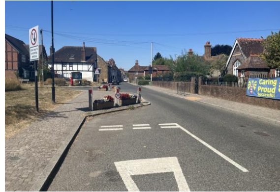
Planters can help soften traffic calming features (Cobham)
