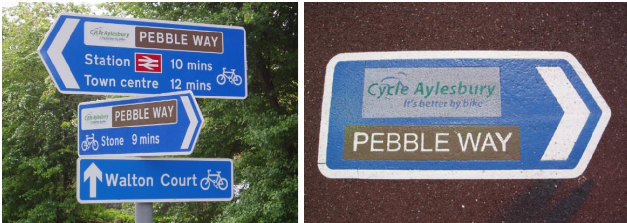
Figure 7.5.5: Left: Signing in Aylesbury showing route branding and local destination off the main route. Right: Thermoplastic marking used only off-highway
